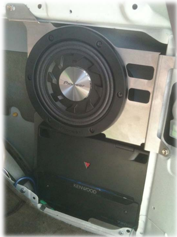
Figure 8. Final mounting of the FJ80MONO Mount in the body panel space with the amplifier and 8-inch sub woofer installed.
