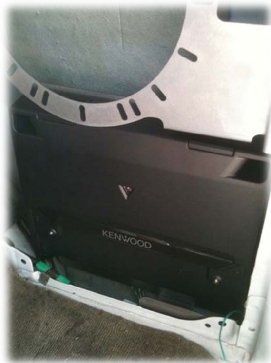
Figure 7. Test fitting the FJ80MONO Mount in the body panel space with the amplifier installed. Take this time to think about where you want to route the wiring for the amplifier.
