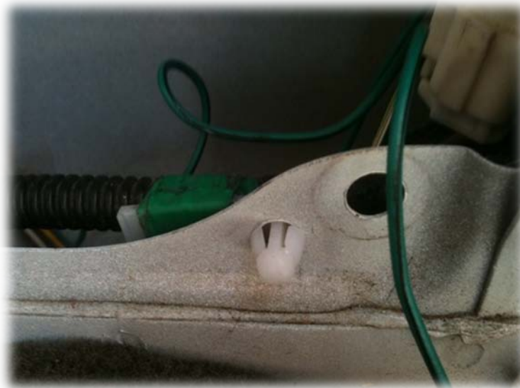
Figure 4. Detail of the factory wire loom clip. To release, simply pinch the tabs and push. After releasing the clip, the loom is free to move around to accept the new mount.
