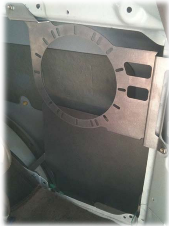
Figure 5. Test fitting the FJ80MONO Mount in the body panel space. Take this time to look at where the factory wires sit and where you want to tie off your new amplifier wiring. In this picture, the factory hardware secures the mount.
