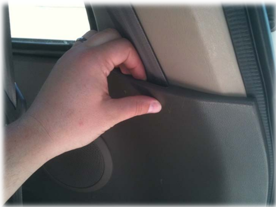
Figure 1. Starting to remove the factory cargo panel. The opening near the rear seat belt is an easy place to get a hold of the plastic. This is easiest to do on a day when the sun has heated up the plastic a little bit.
