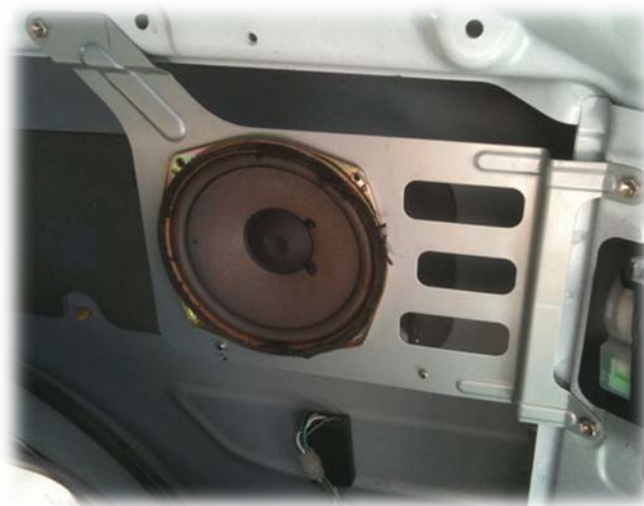
Figure 3. Detail of the factory sub woofer and amplifier that will no longer be needed. Using a 10mm socket, remove the panel and hold onto the factory hardware for your new panel.
