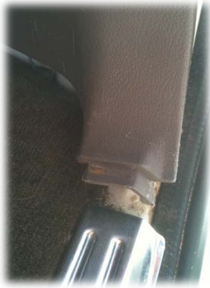
Figure 2. Detail of the body panel tab that mounts under the tailgate trim plate. Once the clips are snapped out of the body, simply rotate the panel towards you to remove it.
