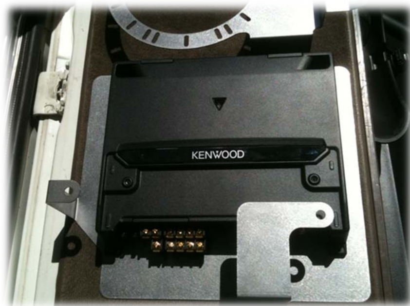
Figure 6. Position the amplifier on the mounting pad. The upper left corner is the most accessible, so the closer to that location the easier your installation will be.
