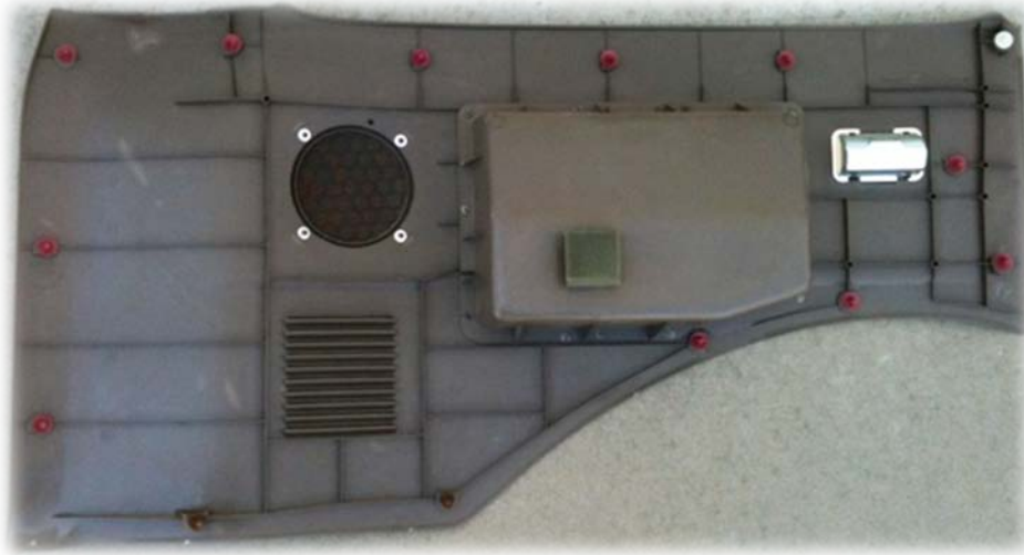
Figure 9. Mounting clips on the factory interior trim panel. For this mount, the stock cubby can be left in place. A perfect distraction for would-be thieves.
